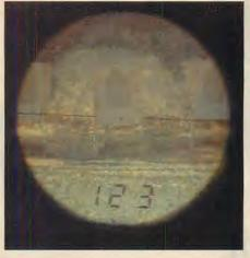
Instantly, the precise range to target is displayed at the bottom of the reticle. This information is simultaneously stored in the system's computer and relayed to the onboard digital inclinometer.
